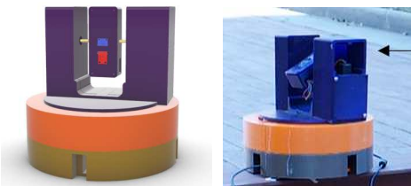
Fig. 7. Terrestrial Laser Scanner developed at the School (Virtual and Physical)
