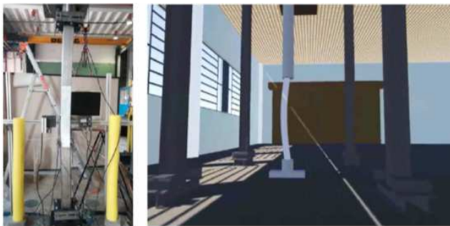
Fig. 10. Virtual reality reproduction of a test using real time measurements.
